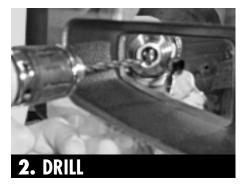
stainless steel insert piece and position into the corner section of the bumper. Note: Front shown in photo at left—Rear shown in photo at right.
